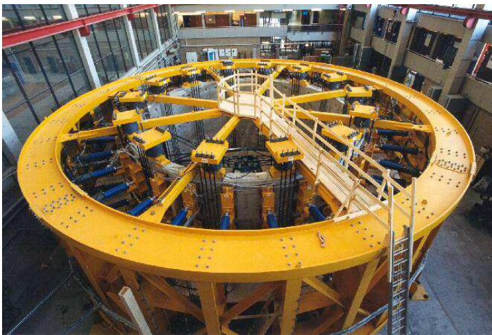
Figure 6 The full scale tunnel lining test facility with 3 full rings
